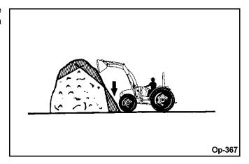
Another method for large dirt piles is to build a ramp approach to the pile.
